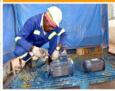
SUBMERSIBLE PUMP REPAIRING
